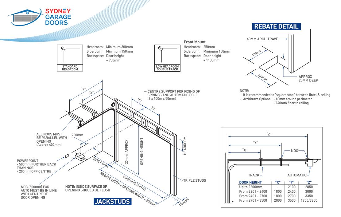
We recommend square stopping gib at lintel as Gib Cove can interfere with spring/automatic fixing. If Gib Cove used it may require notching out which can look untidy.
